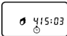
2. Press the key
