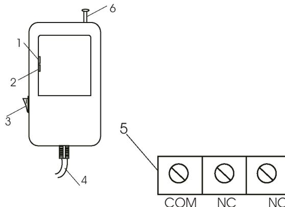
1. Receiving the signal from the transmitter indication- green LED
