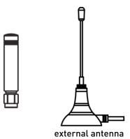
Caution! In case, if the distances between Euroster C6 system devices are significant we recommend using an external antenna (with a magnet, to be installed on the outside of the distributor cabinet).
